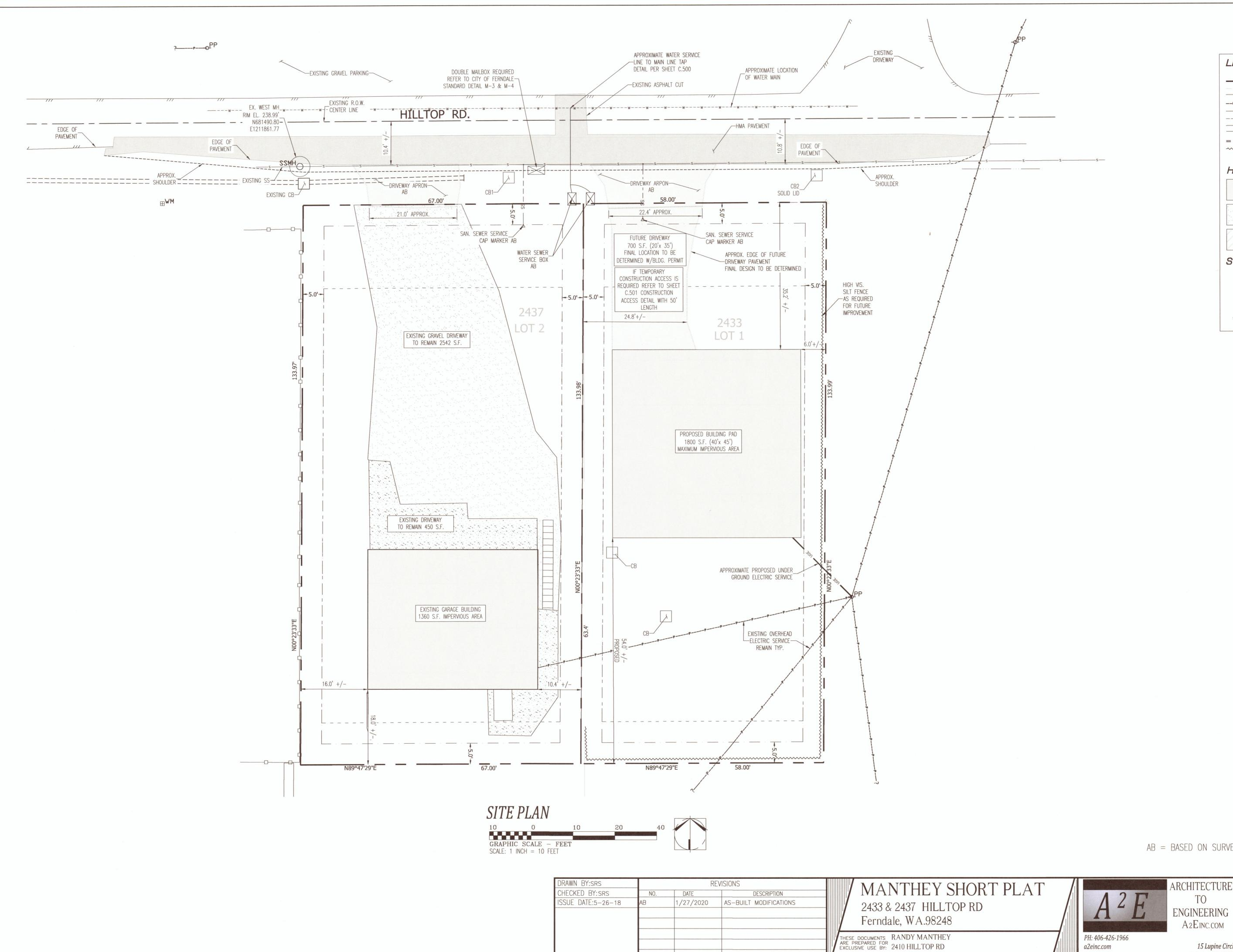
LINE LEGEND = 5 FOOT SETBACK LINE = CHECK DAMS PER SHEET C.501 (WSDOT STD PLAN I-50.20-01) HATCH LEGEND = PROPOSED/EXISTING BUILDING & DRIVEWAYS AREAS = EXISTING GRAVEL SURFACING = PROPOSED STORMWATER DISPERSION FIELD, REFER TO SHEET C.300 SYMBOL LEGEND EXISTING TREES/STUMPS WV WATER VALVE EN WATER METER AFH FIRE HYDRANT SANITARY SEWER MANHOLE
