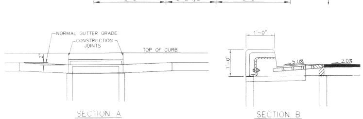
THRU-CURB INLET FRAME + GRATE WITH VERTICAL CURB INSTALLATION NTS
